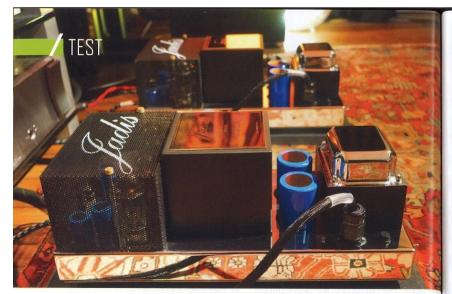
1 to 16 ohms by a set of strips that configure the secondary windings of the lifetime guaranteed output transformer. It will therefore be necessary to open the device to switch from 4 to 8 ohms for example.
