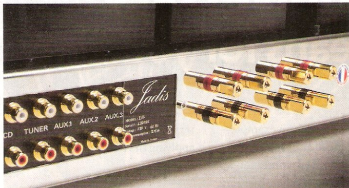
The Jadis provides five line-level inputs and two sets of unlabeled binding posts.
